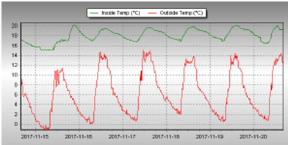
Data from my weather station: inside (green) and outside (red) temperatures. On the 15th of November 2017 the wood stove was lighted because of cloudy cold weather. Then the sun started to shine and was able to maintain temperatures around 19°C inside without the stove.
